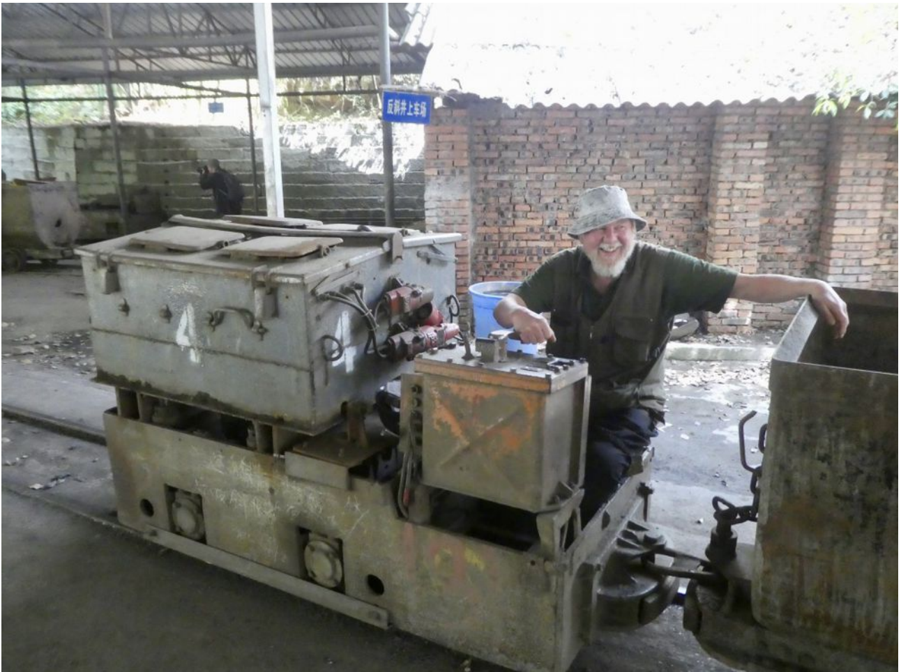
Shibanxi is not just about steam tourist trains - this is one of several battery electrics working the spoil at the back end of the Sanjin mine.
