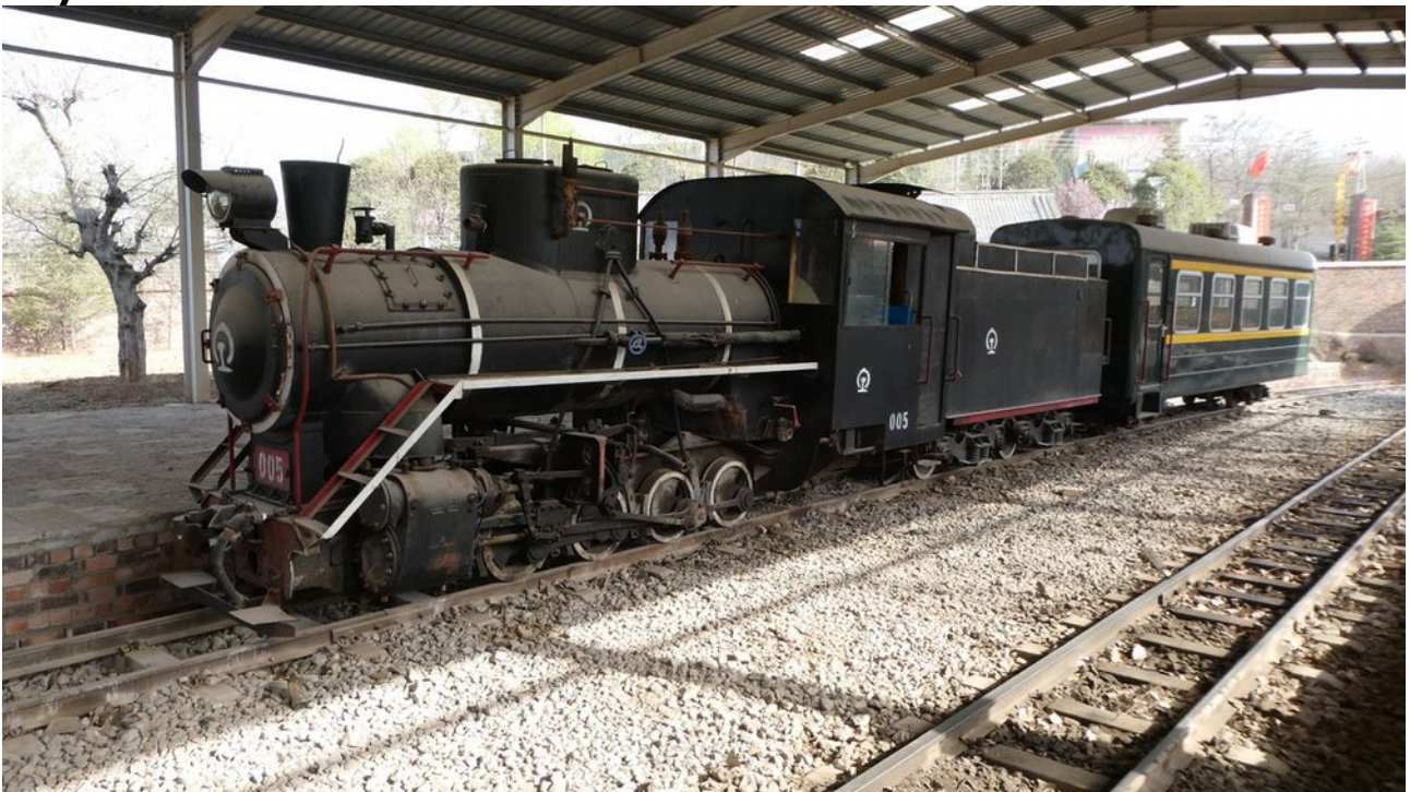
C2 005 with a single coach at platform 2 at Chaoyanggou. It displays some changes including a new low chimney, altered smokebox door, various new bits of steel plate and water feed pumps instead of injectors.
