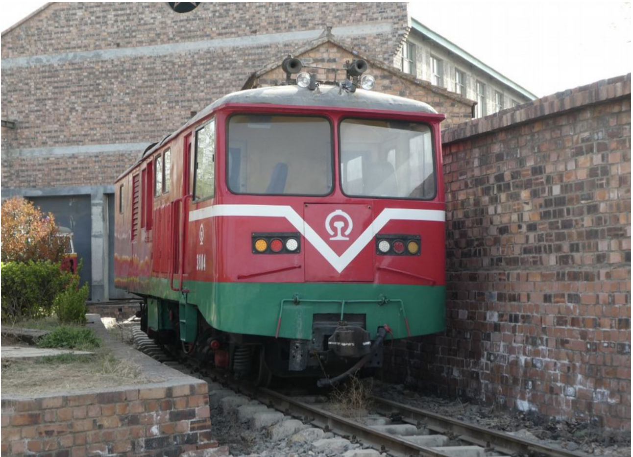
JMY380 3804 at the depot has a cab at one end only.
