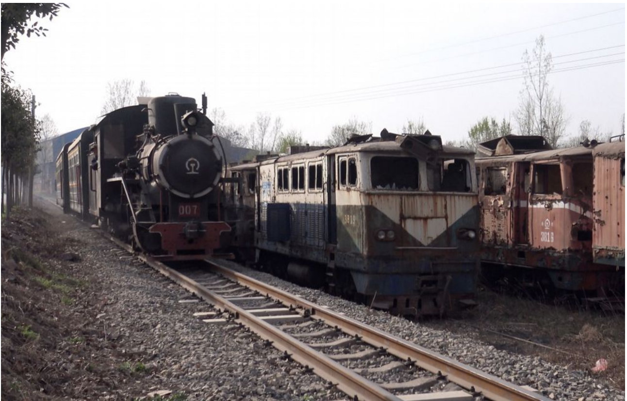
Unfortunately, 007 and other C2s here have been adapted with noisy diesel generators in the tender. One of the purposes for this is to feed water into the boiler in place of the original steam injectors.
