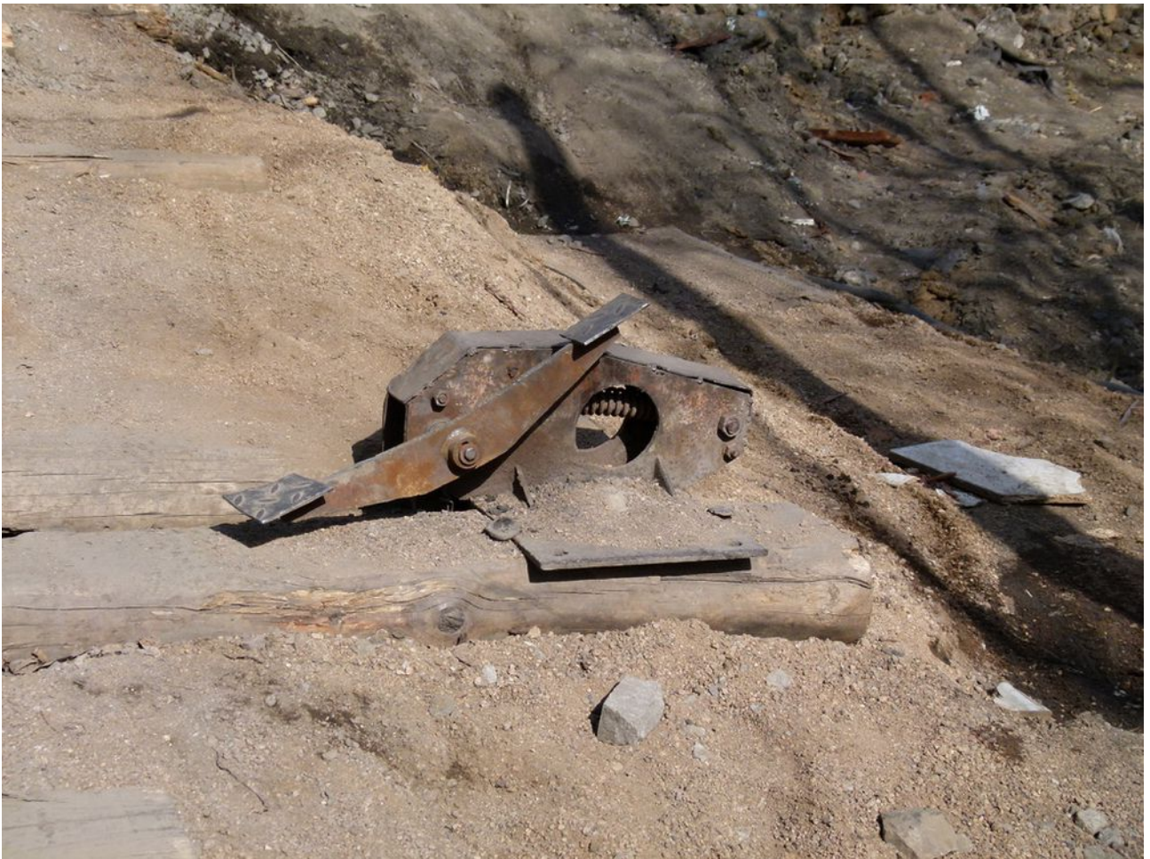
Points operated by a foot treadle. ©Mike Jackson, 2019
