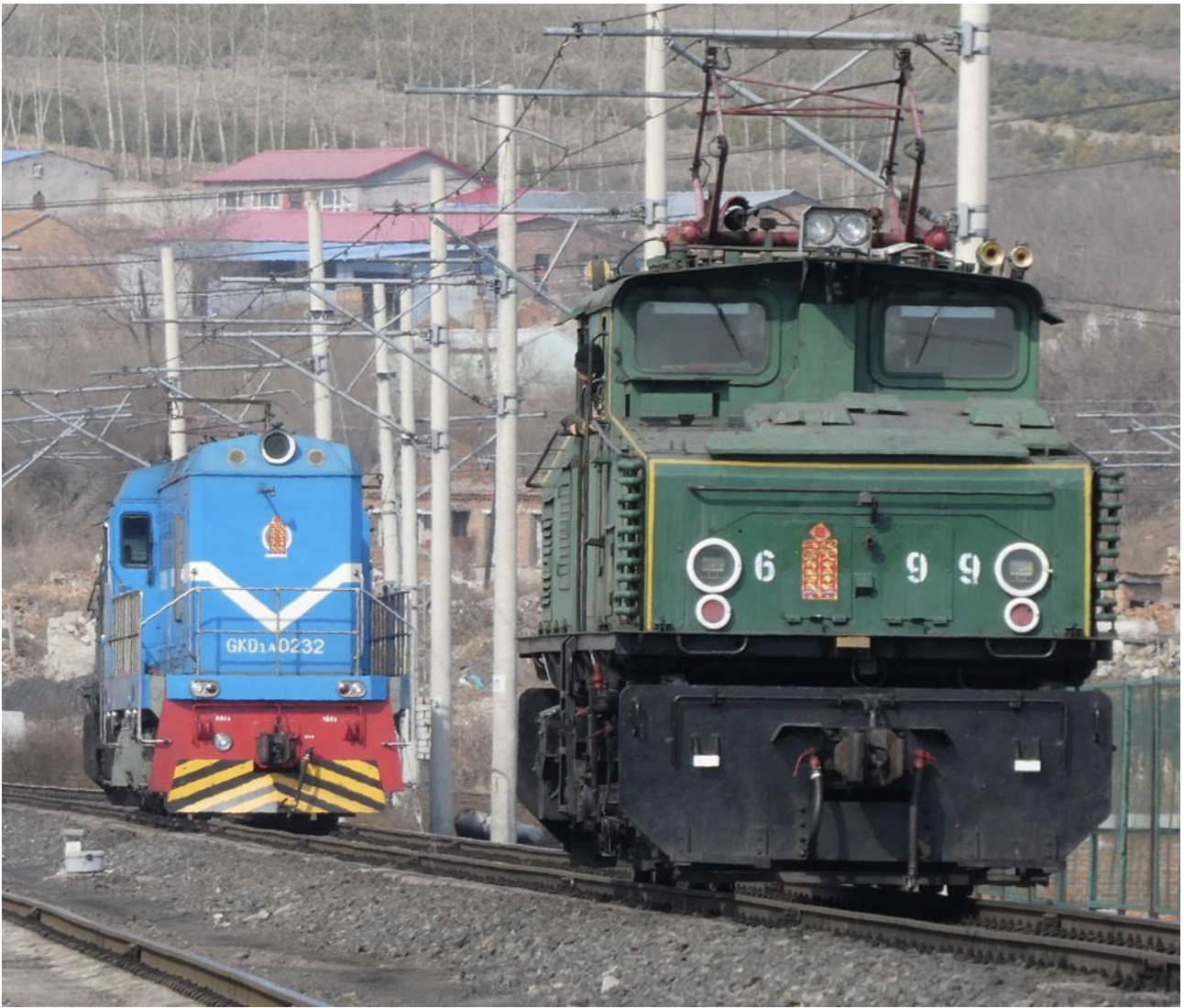
Electric 6399 along with diesel GKD1 0232. We didn't work out the diesel's role on this electrified system.
