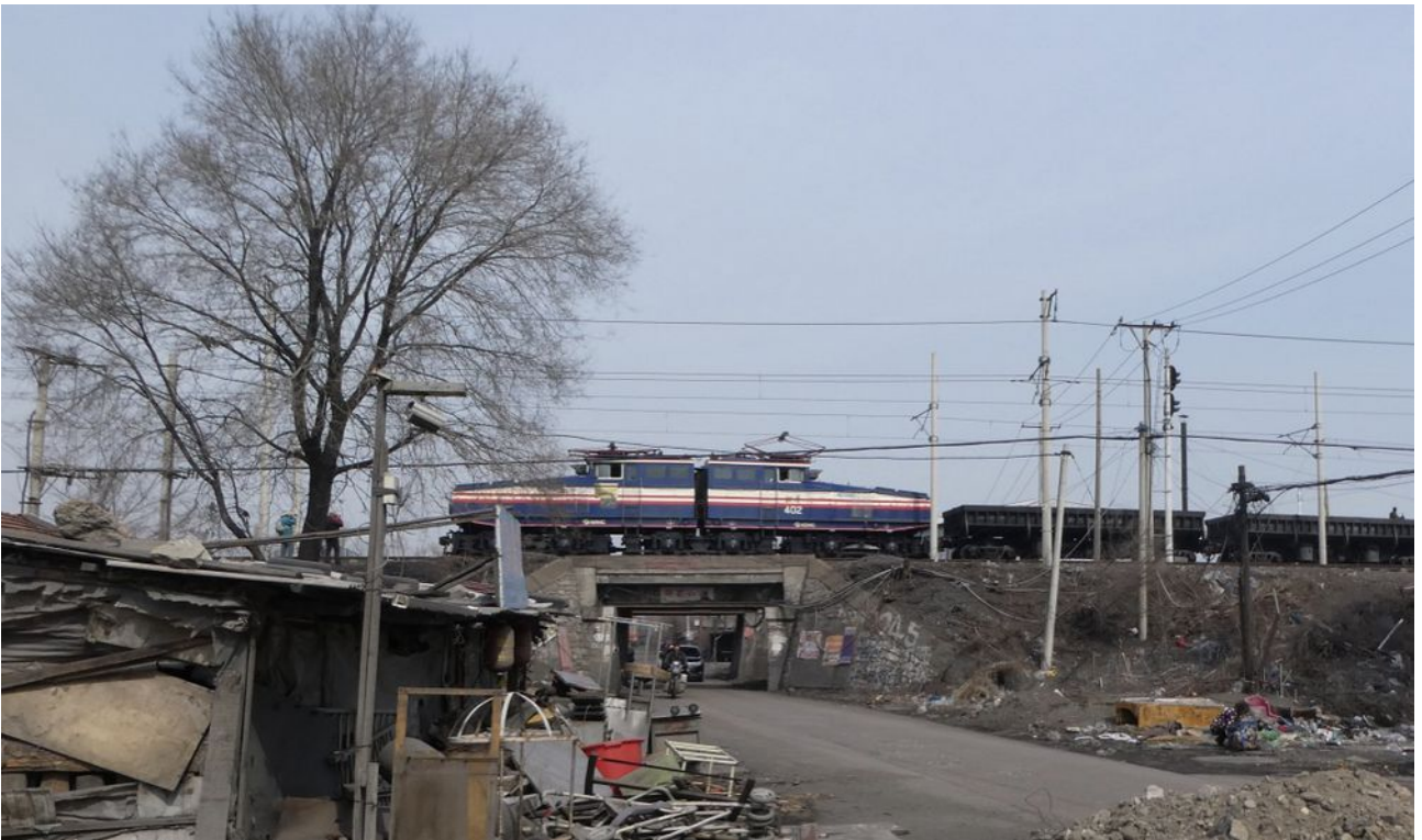
Most unusual was twin unit electric ZG150-1500 402 one of two allocated here. The two units have a shared bogie in the middle.
