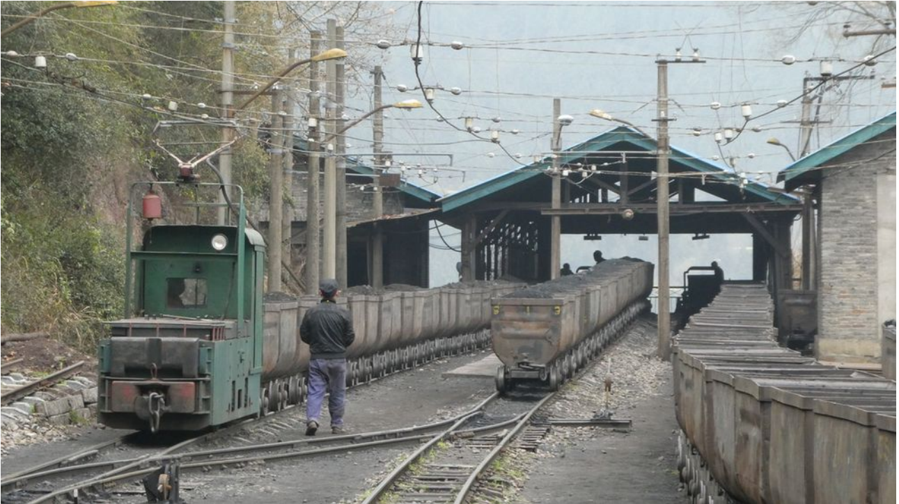
Full tubs on the left are tipped with a front end tipper and moved to the empty tub lines on the right.
