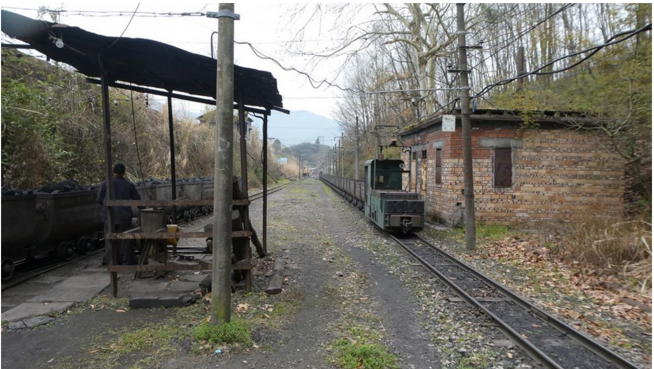
With spoil tipping proceeding, a train of empty tubs returns to the mine.
