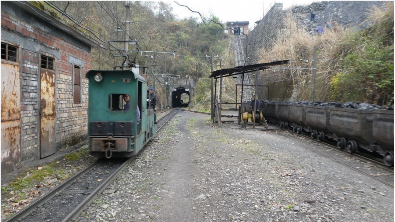
This loco has delivered spoil to be hauled up the incline and tipped.
