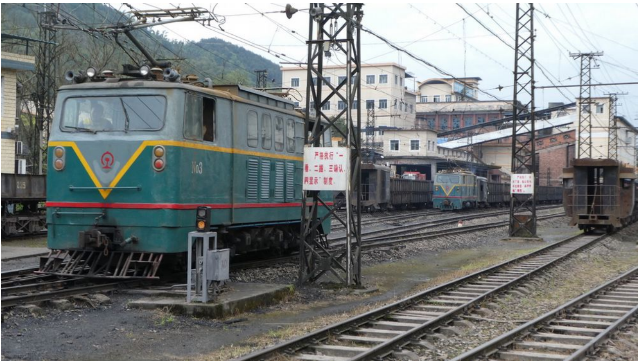
Two locos and two cabooses in the yard at Honglu. On the left a bogie caboose and on the right a 4-wheel version. The bogie versions are use on the section to China Rail.
