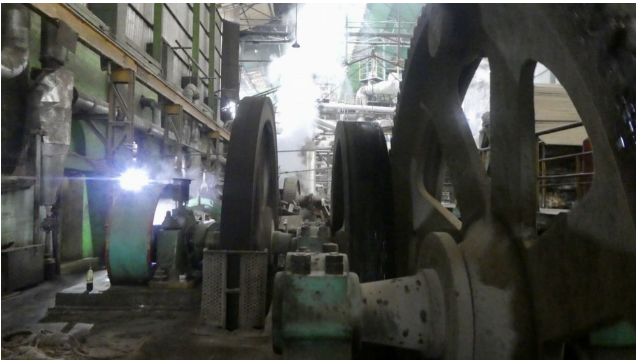
Two steam engines survive near the beginning of the mill train and these are larger engines than those at Olean and Wringinanom.
