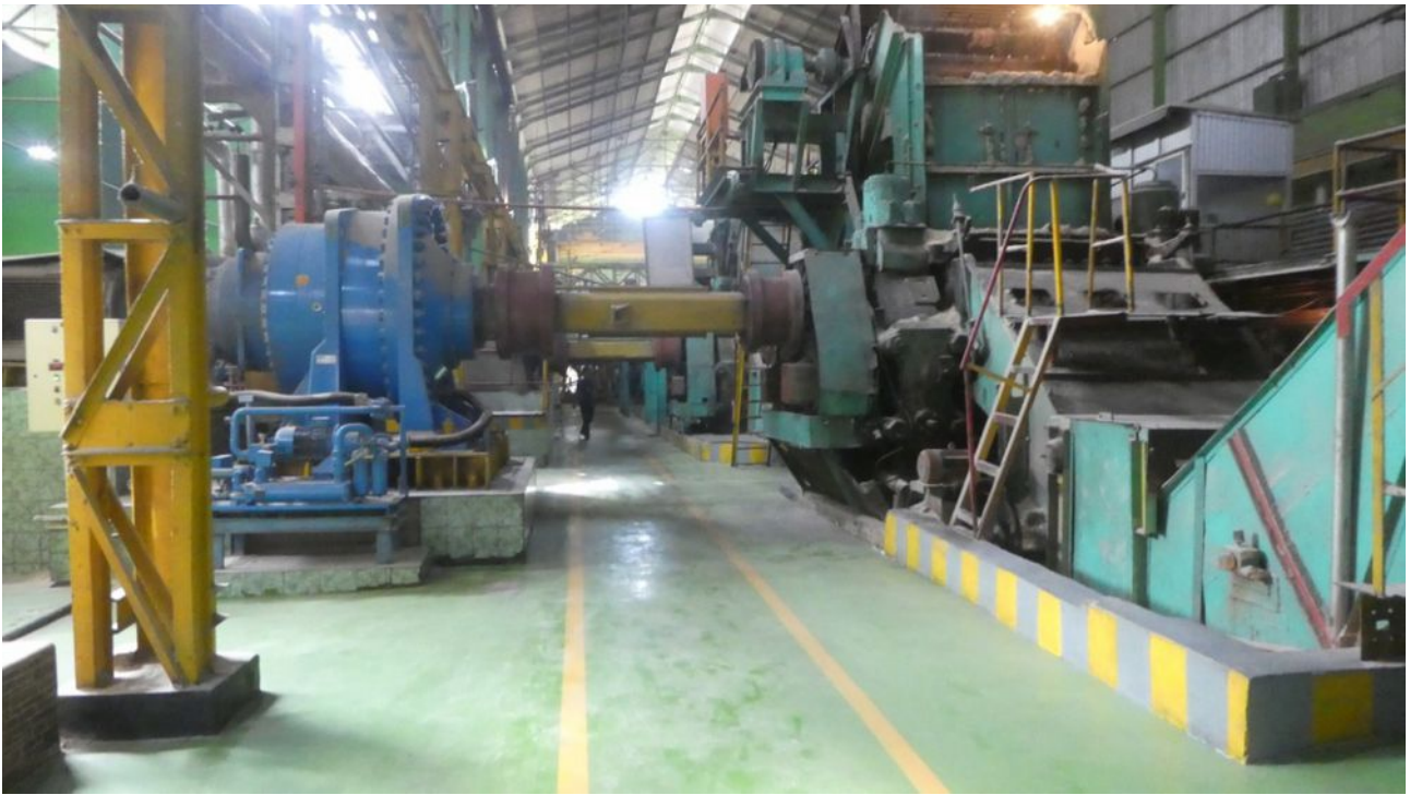
The blue item on the left is an electric motor, two of which have replaced steam engines powering the mill train.
