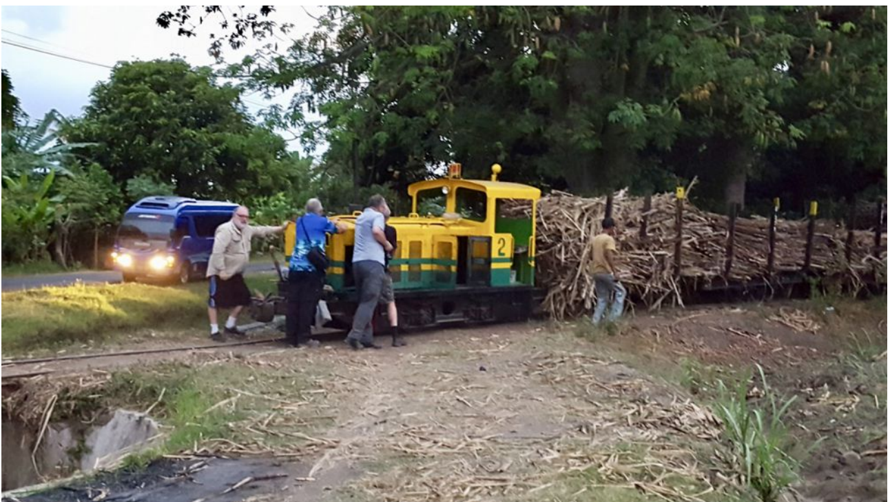
The tractor could not cross the railway bridge due to the gauge of its wheels so it pushed the loco forward and ran round to the other side on a road bridge. No. 2 needed to be pushed back and coupled up to the train prior to a cable being attached so the tractor could pull the train across the railway bridge. The 'turiis' lent a helping hand (from left, Ross, me, Chris and Graham).
