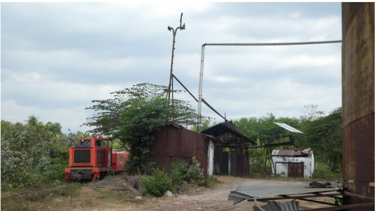
This is the unloading facility. The molasses are dumped out the bottom of the tankers and pumped into the tank (visible on the right).
