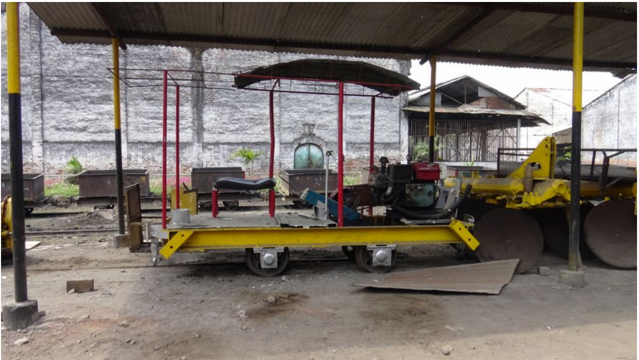
This new 'speeder' built using a Chinese agricultural diesel is outside the loco depot and looks almost complete.
