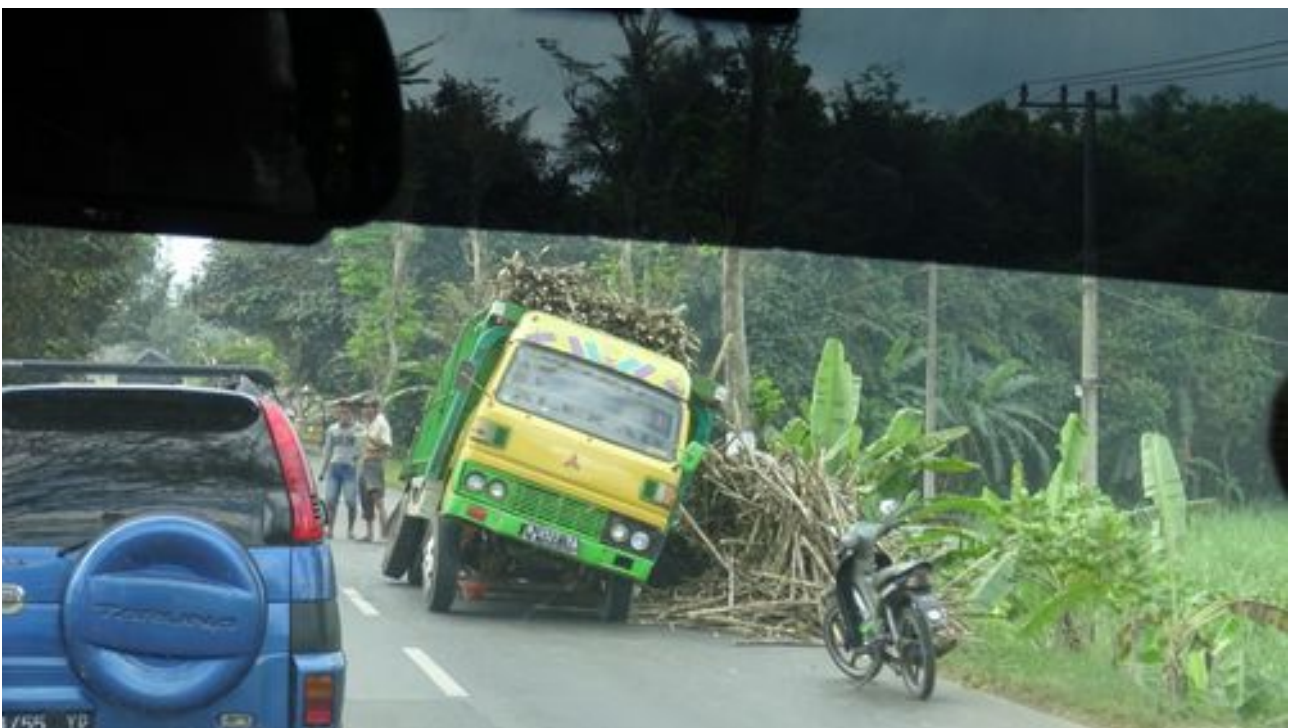
In this case, it would have been better for the cane to go by rail! Truck with a broken back axle seen from our bus on the way to Probolinggo.
