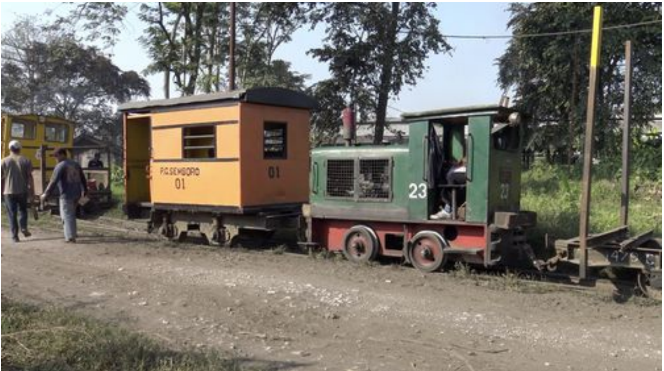
Our 'small diesel' train being assembled. Carriage 01 is used by the Permanent Way crew for re-railing locos or lori and carries big jacks and wood for packing.
