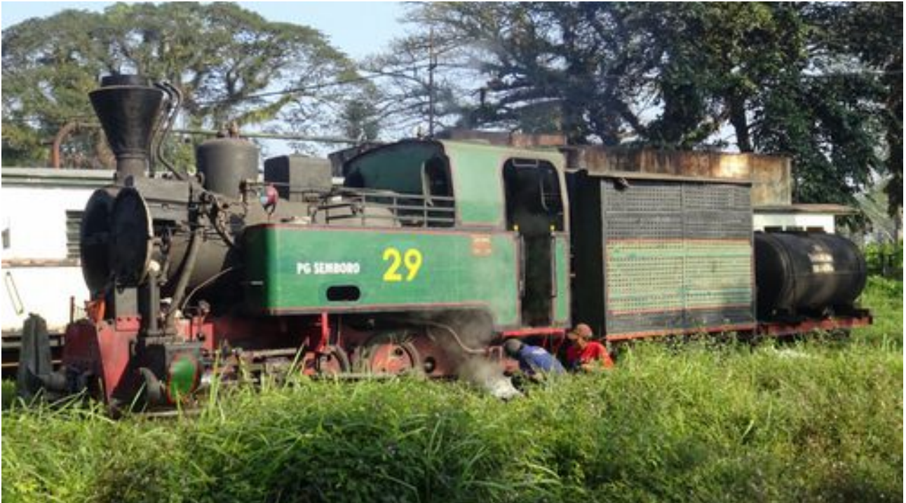
Working on the injector on No. 29. It only has one. They borrowed a replacement off the Mallet but that still didn't do the job.
