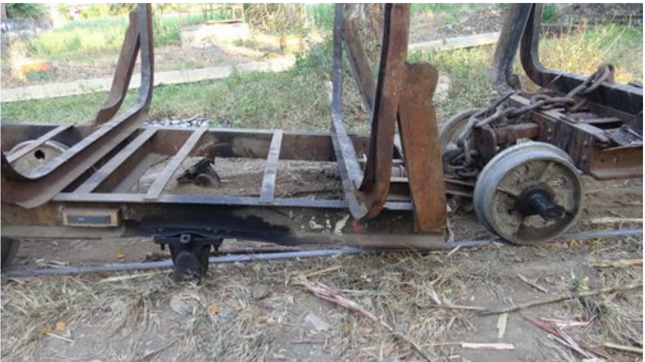
Despite only having tracks inside the mill, the conditions are brutal for the lori. Note the two axle boxes centre right (far one half detached) and the axle and wheels now between the lori (right). The lori now all have a RF ID strip (seen left of near axle box) which allows the whereabouts of lori and its load to be recorded and could be use to keep payment and other records for the truck
