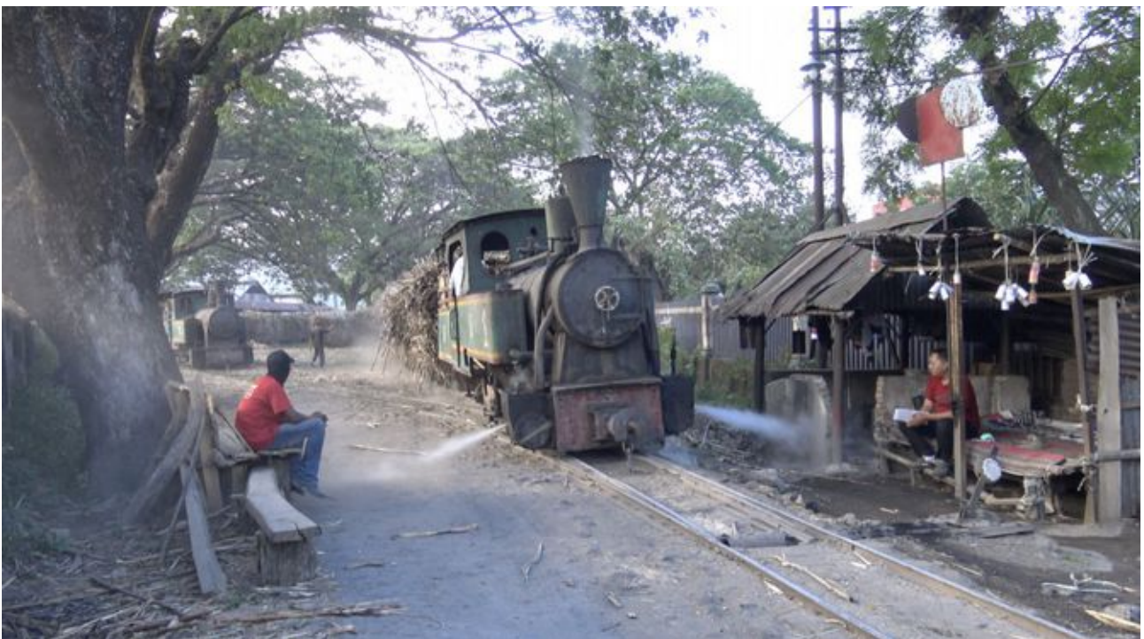
Reminding me of a scene from years ago, perhaps assisted by the overcast sky, No. 16 propels the loads past the control point at the entrance to the mill yard. The signal (which can be rotated) is top right and shows a white disk for proceed. The red square for stop is achieved by turning the signal through 90 degrees.
