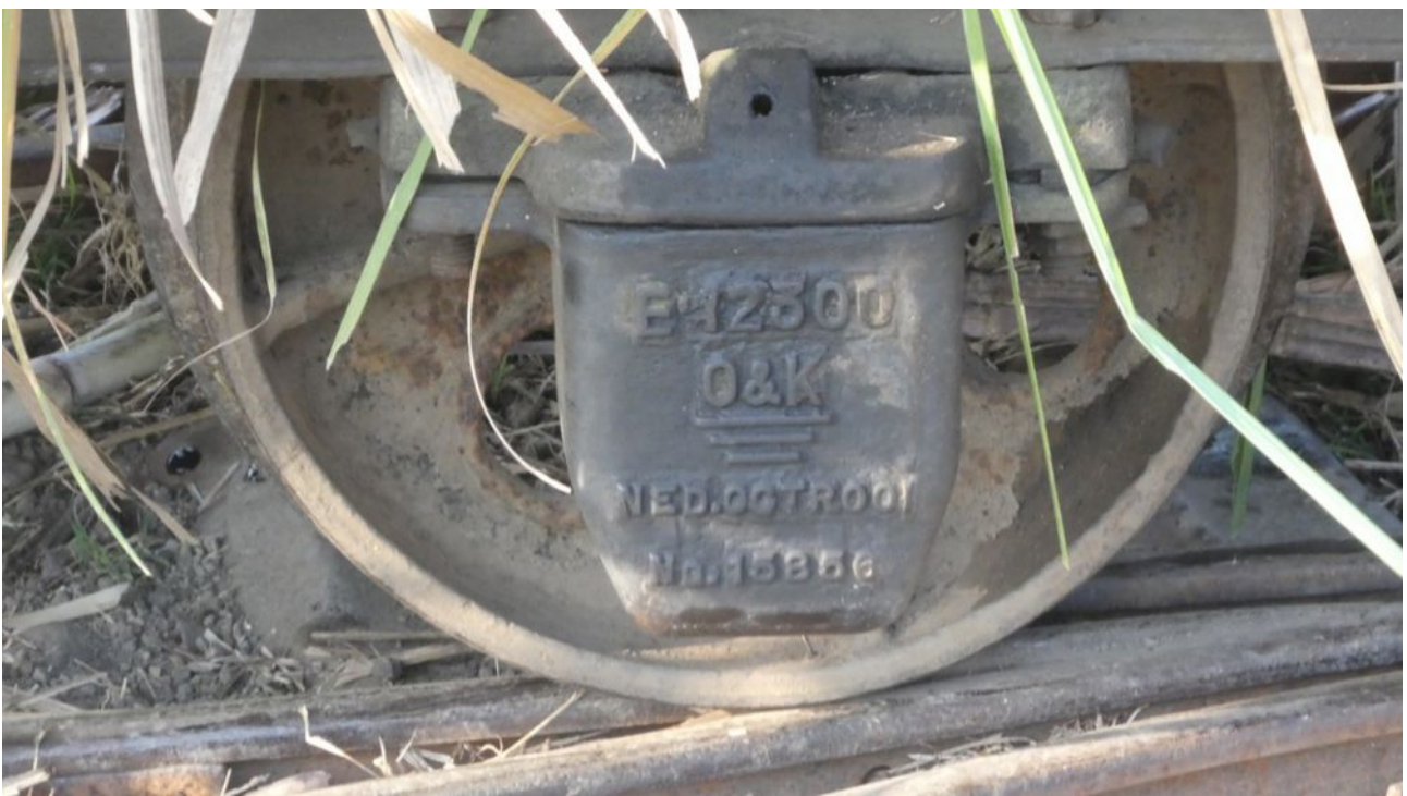
One of the axle boxes is labelled up as a pre-WWII German O&K export to Dutch Indonesia. O&K were the biggest exporter of steam locos to the sugar mills but supplied more besides.
