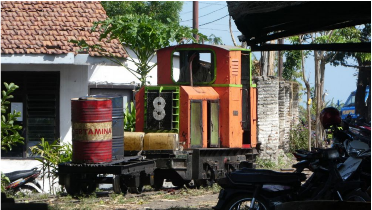
The yard pilot is a British Baguley loco with a Deutz engine.
