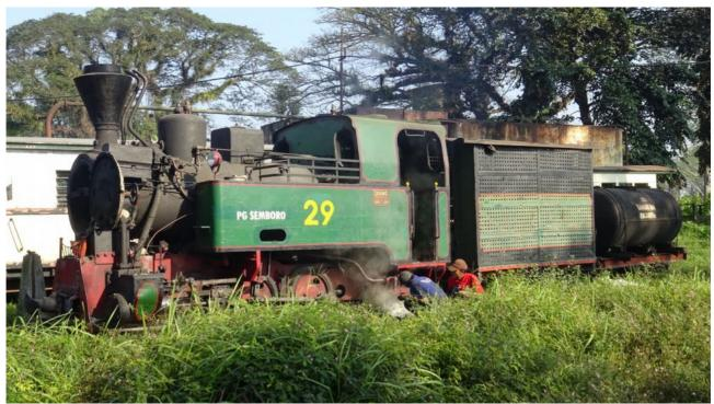
No. 29 in steam but with crews trying to repair the injector. They eventually dropped the fire and lost the pressure so they could work on it properly but to no effect.
