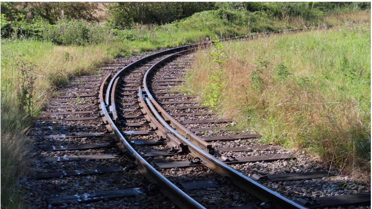
The passive points once needed to operate the dual gauge train round the loop but still used with the 2ft gauge only track.
